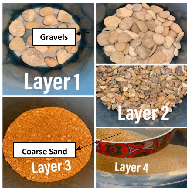
Figure 1: Multiple Layers of Sand were Sand Filtration System.
